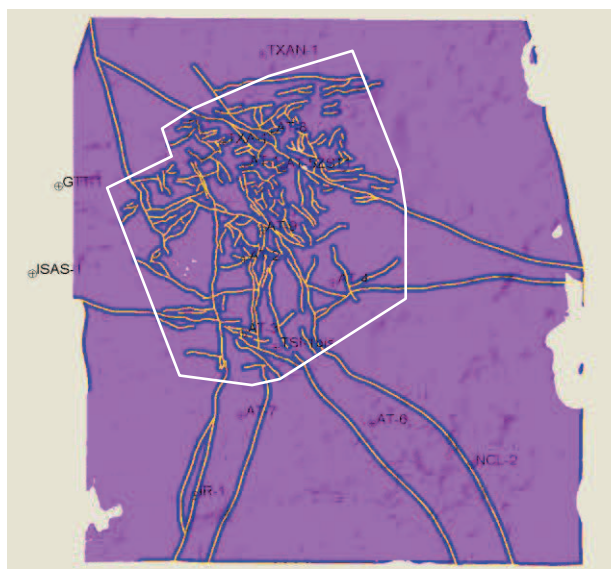
Figure 4-5 Seismically & structurally interpreted fault pattern with 100 m & 500 m fracture corridors
